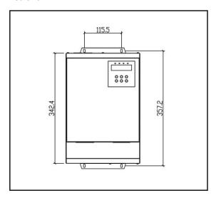
2. Install the unit by screwing four screws. It's recommended to use M5 screws.
